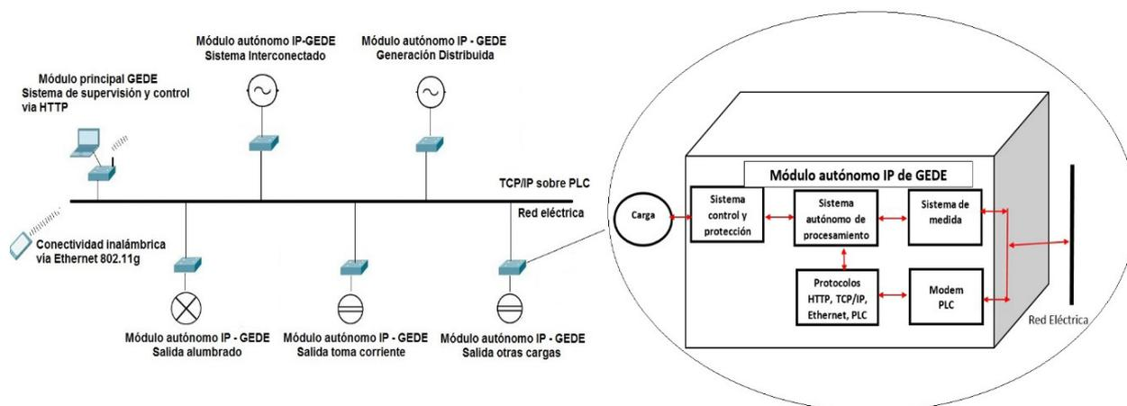
Figure 5: Deployment diagram with communication protocols for GEDE
