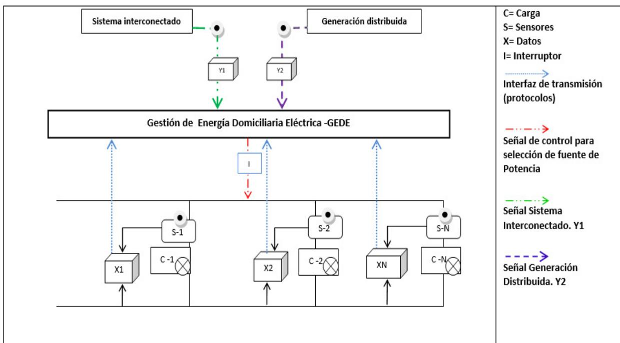
Figure 4: Block diagram of the operation of the GEDE model.
