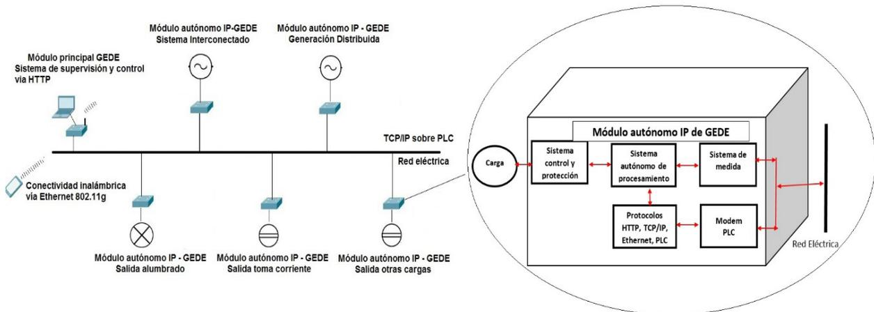
Figure 5: Deployment diagram with communication protocols for GEDE
